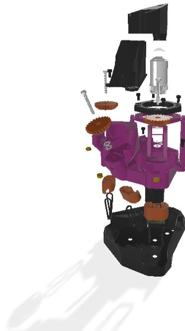
Figure 2.2.4 - Exploded View of the OpenFlexure Microscope
